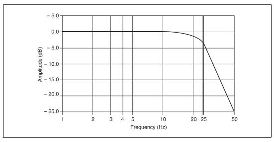
Figure 2. Typical SCC-LP01 Response Curve
